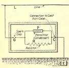
Fig. 157.—The condenser-type protector.
